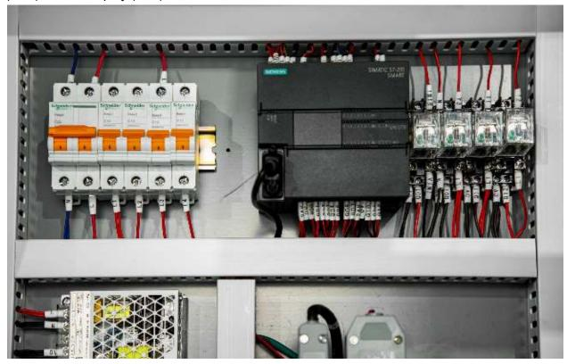
The PLC, which acts similarly to a microcomputer, controls the functionality and functioning of the packing machine. An HMI, which is often a color touch screen measuring between 7 and 12 inches, serves as the interface through which a person may make changes, get feedback, and obtain updates.
