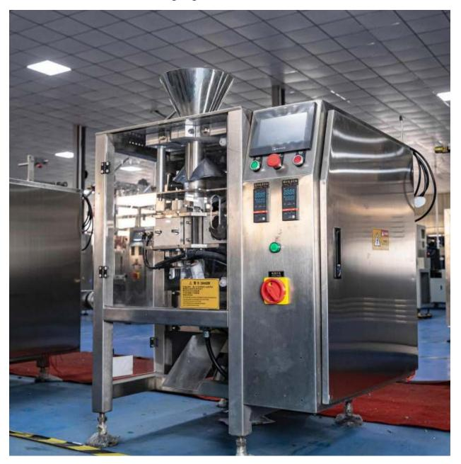
On the other hand, <u>vertical packaging machines</u> are designed to work with <u>powdery</u>, granular, or liquid products in form. These items need to be packaged in a way that will ensure their stability and prevent them from leakage.
